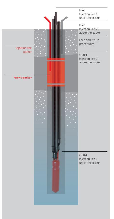
\*An Artesian well or an Artesian feed arises if drilling is carried out in a groundwater bearing layer with an hydraulic potential that is high enough to rise up to the surface of the ground, or higher, on its own, i.e. without pumping. The *GEOtight*<sup>®</sup> fabric packer was developed by Swiss drilling engineers and geologists; on site from professionals to professionals on site.
