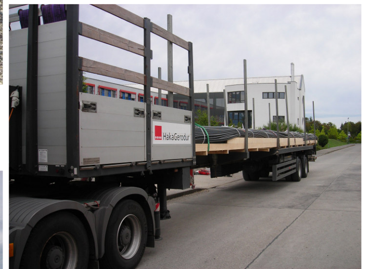
Special transporter for 20 m geothermal pile probes
