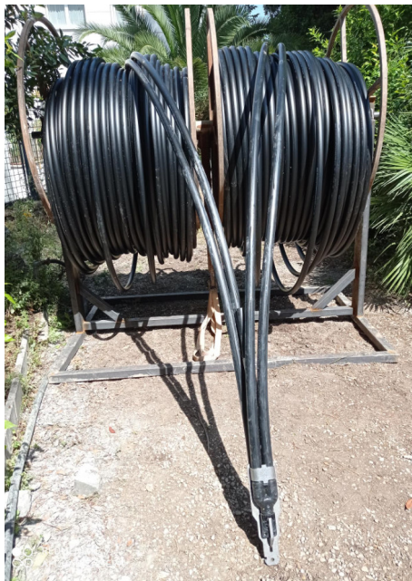
Image 5: VARIO probe with PUSH-FIX installation aid Source: Georicerche Srl
